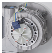
Gear box protection (hall effect)
